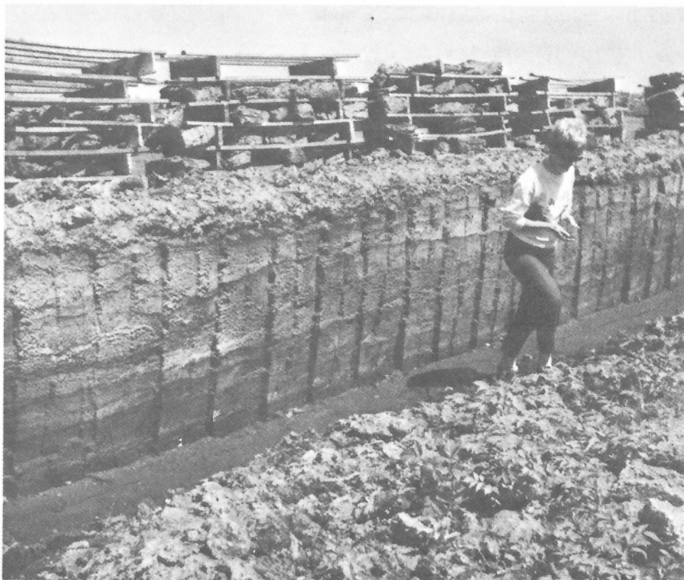
Plate XV. Cutting in peat bog; the excavated moss is placed in racks to dry. Fafard Peat Moss Company Limited.
