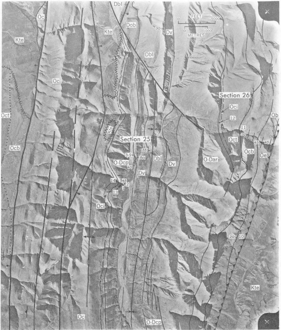
Figure 3. Vertical aerial photograph of Sections 25 and 26, west of Irene Bay, Ellesmere Island. The type section of the Vendom Fiord Formation (Dv) is in Section 25. Symbols - Ob, Baumann Fiord Formation; Oe, Eleanor River Formation; Oc, Cornwallis Group undivided; Ocb, Bay Fiord Formation; Oct, Thumb Mountain Formation; Oci, Irene Bay Formation; O-Dar, Allen Bay and Read Bay Formations undivided; O-Dcp, Cape Phillips Formation; Dv, Vendom Fiord Formation; Dbl, Blue Fiord Formation; Dob, Okse Bay Formation; Kte, Eureka Sound Formation - Barbed line, thrust or reverse fault; heavy line with dot, normal fault with dot side down; jagged line, angular unconformity.
