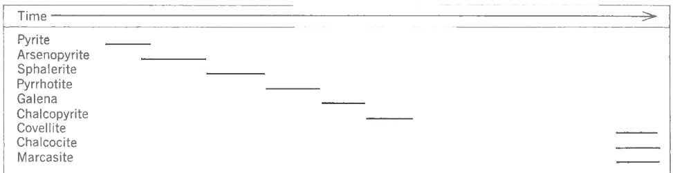
Figure 6. Paragenesis of the Middle River, Anacon Lead Mines (New Larder "U") and Anaconda (Caribou) orebodies
