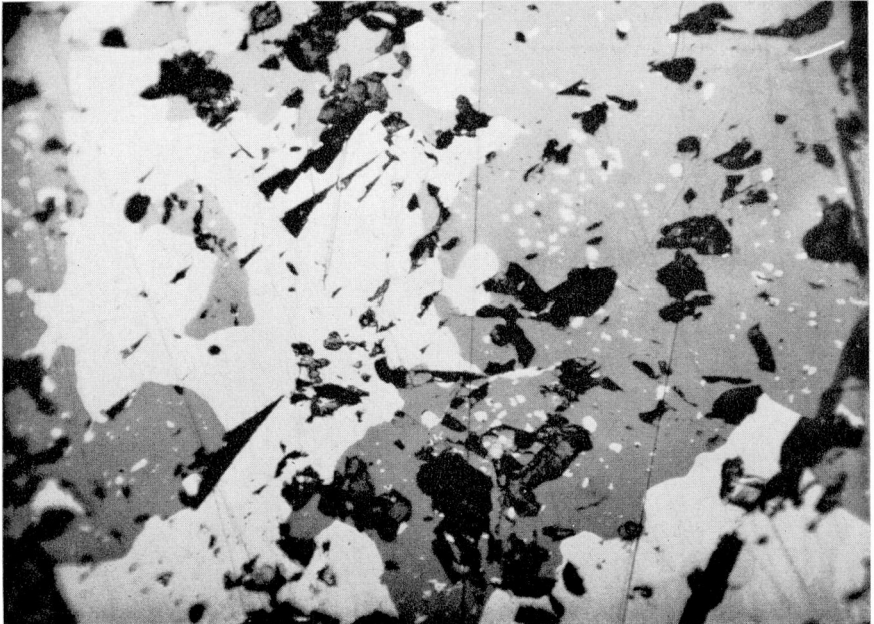
B. Second generation chalcopyrite (white) replacing sphalerite (grey) containing exsolution blebs of first generation chalcopyrite (white blebs), Nigadoo orebody. x200
