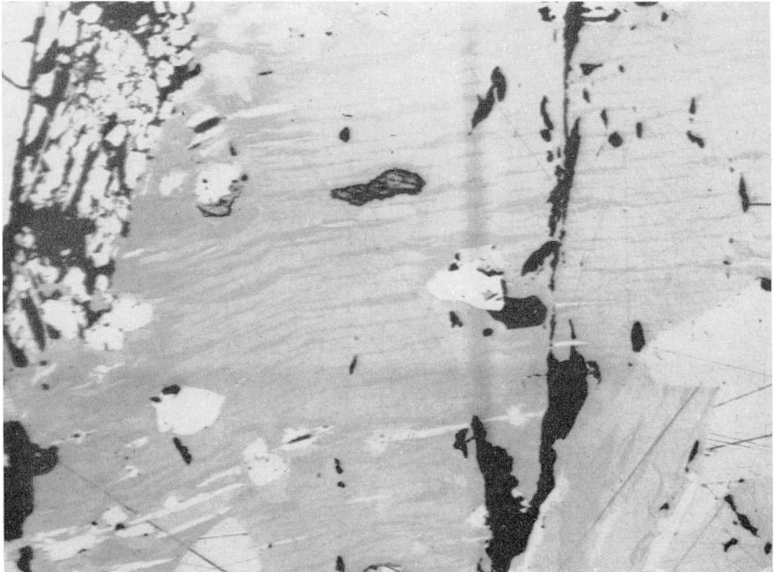
B. Chalcopyrite-tetrahedrite exsolution intergrowth. Curved lamellae of tetrahedrite (darker grey) in chalcopyrite (pale grey) host. Nigadoo orebody. x400
