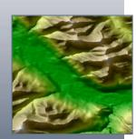
A digital surface model (DSM) is a digital representation of elevations captured at the top of features such as treetops or building roofs. CDSM elevations are derived from radar interferometry data captured during the Shuttle Radar Topography Mission (SRTM) performed by the space shuttle Endeavour in February 2010.
