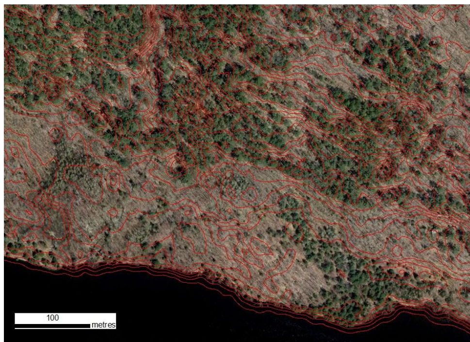
Figure 4 Aerial image and HRDEM contours.
